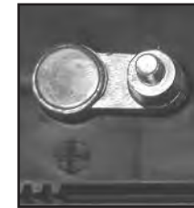
POSITIVE POST HAS LARGER DIAMETER
