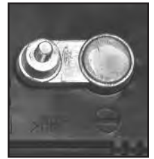
NEGATIVE POST HAS SMALLER DIAMETER
